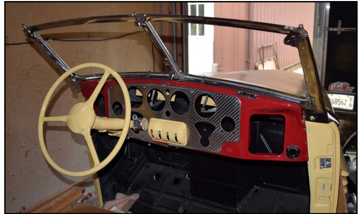
Our 1936 Cord Convertible Phaeton Sedan is coming along slowly. The re-plated windshield frame, Ramada Red instrument panel and new gauge panel are done.
