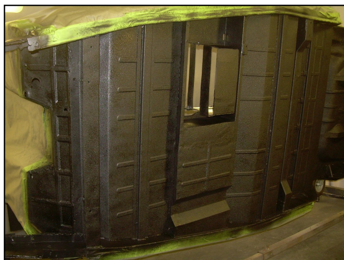
The underside of the Cord body was sprayed with black pickup bed liner material which is virtually indestructible. This replaced the original black undercoating that had been applied when the car was built at Connersville.
