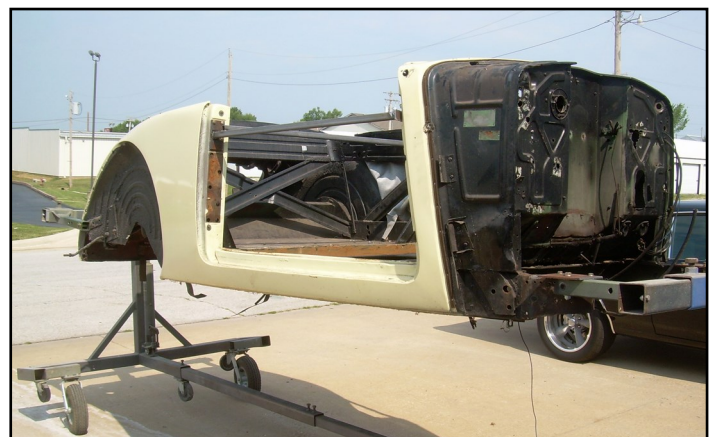
This is the picture we saw on Tuesday after the Cord was delivered to Buffalo on the previous Thursday. Note the 1" x 1" steel braces in the totally stripped body.
