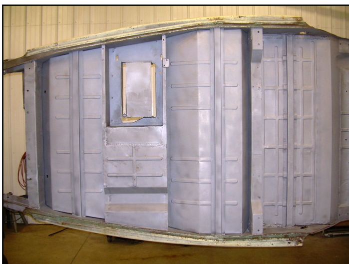
The 1936 Cord after all new pressed steel floor pans were welded in place by the guys at Buffalo Paint & Body. Everything is almost perfect at this point.
