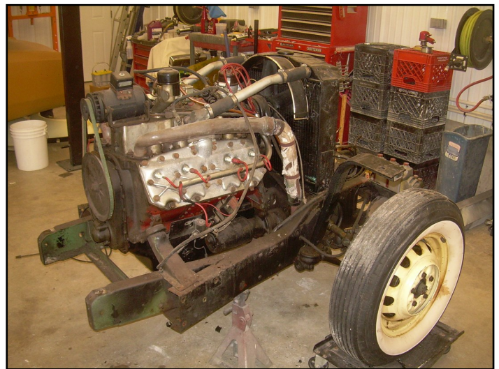
The entire front sub-frame had to be removed to properly restore the underside and structure of the 1936 Cord 810 body. It is held together with twenty bolts.
