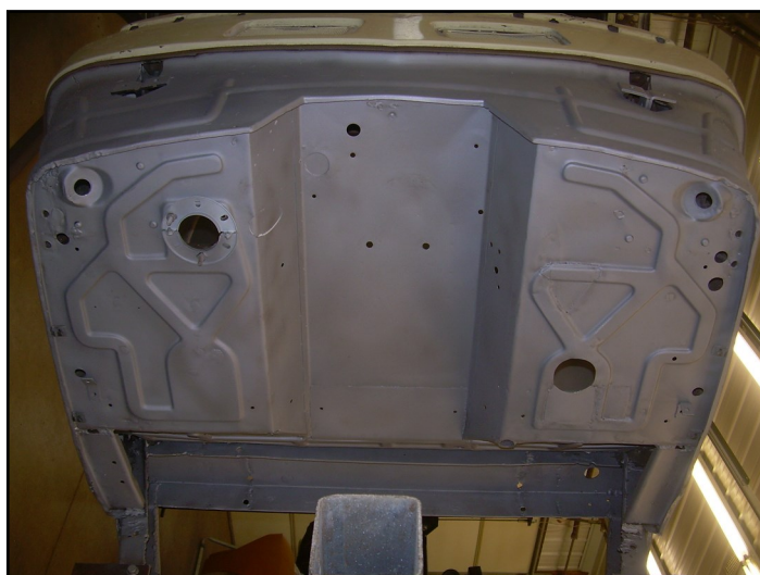
While the body was disassembled we told the guys at Buffalo to repair and restore the firewall according to detailed drawings were got from Stan Gilliland in Kansas.
