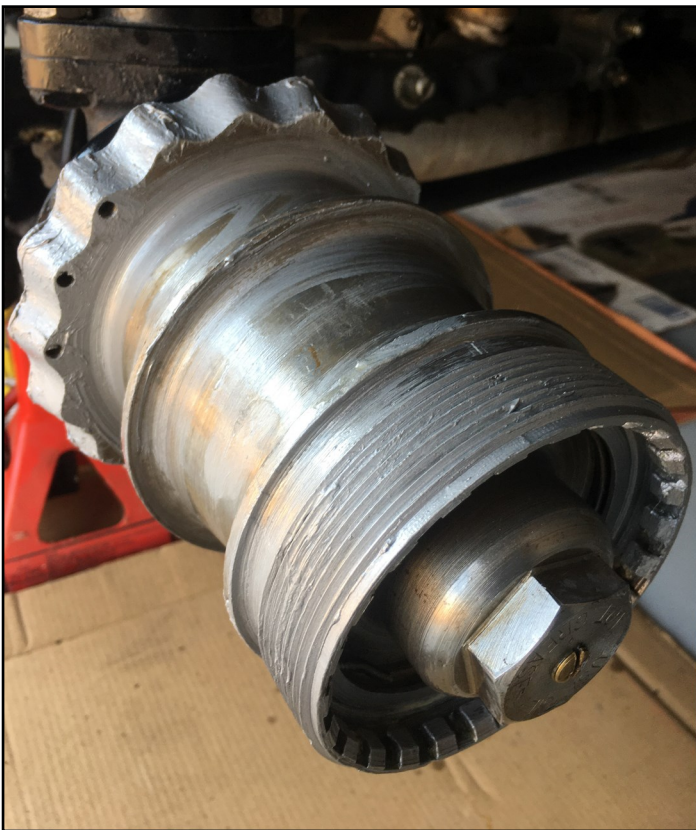
Buffalo hub cleaned and ready for installation.
