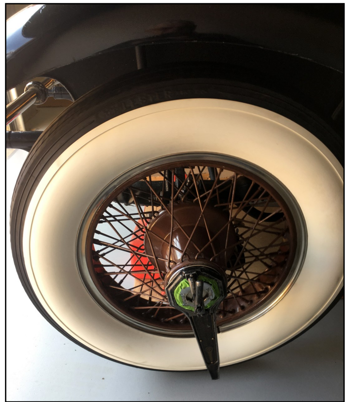
The Rolls-Royce Buffalo wheel with special hub wrench and locking lever in place. A similar wheel and hub assembly was used on Classic 1926-1929 Cadillacs and Model J Duesenbergs.
