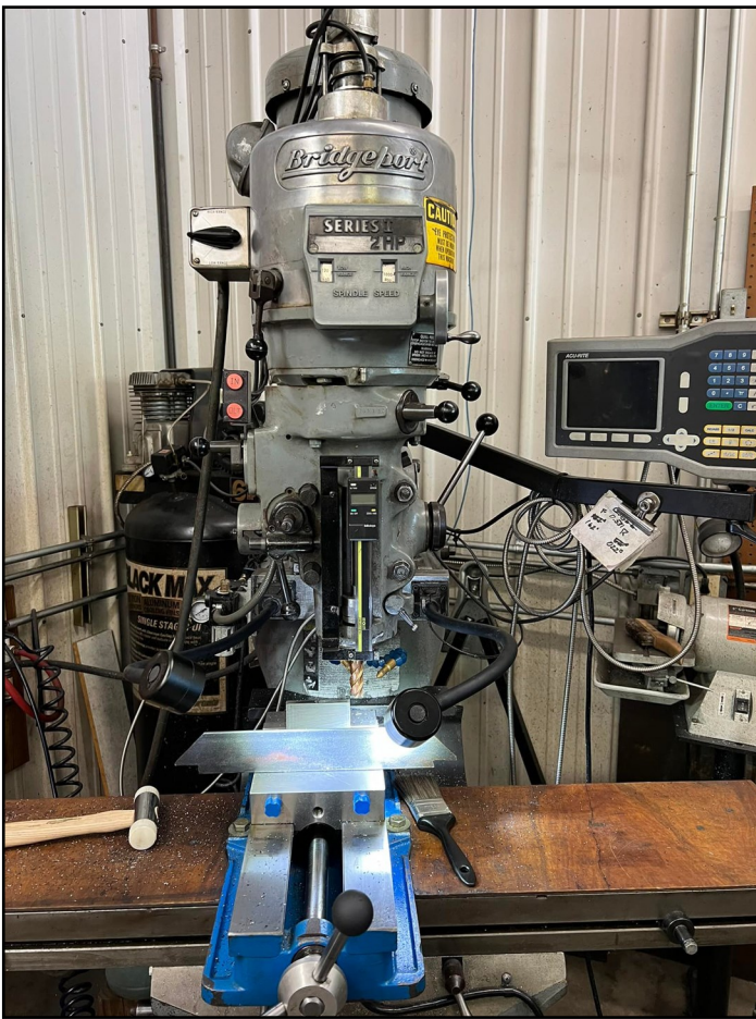
This massive multi-purpose machine is called a "Bridgeport" and is the ultimate dream of any machine shop. Its operation is obviously complicated and part of any good machinist's training.
