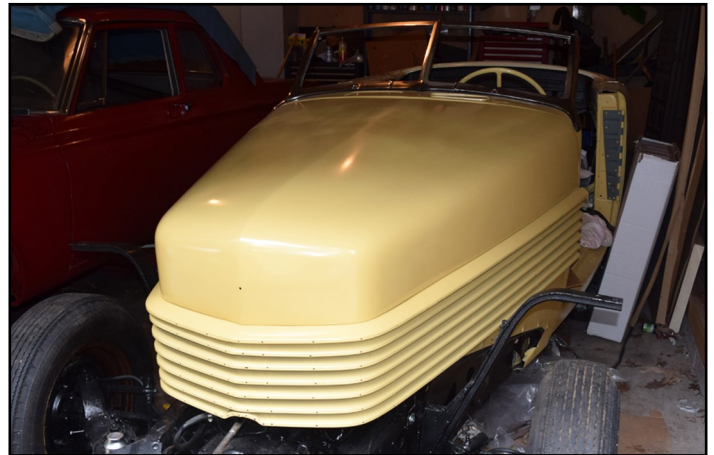
Paint work has been accomplished on the fender and hood of our 1936 Cord 810 Convertible Phaeton.
